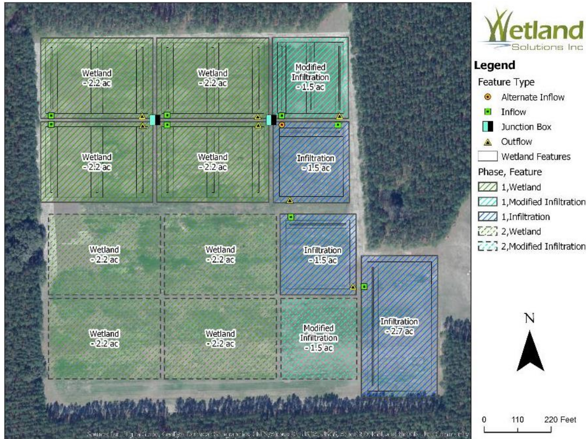
Figure 8. Proposed High Springs Wetland Layout
