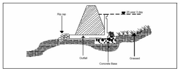
FIGURE 19 Retention basin design (SFWMD 2002b)
