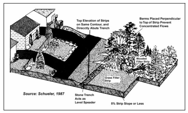
FIGURE 17 Buffer strip design (SFWMD 2002b)
