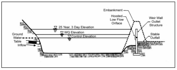
FIGURE 18 Wet detention pond design (SFWMD 2002b)
